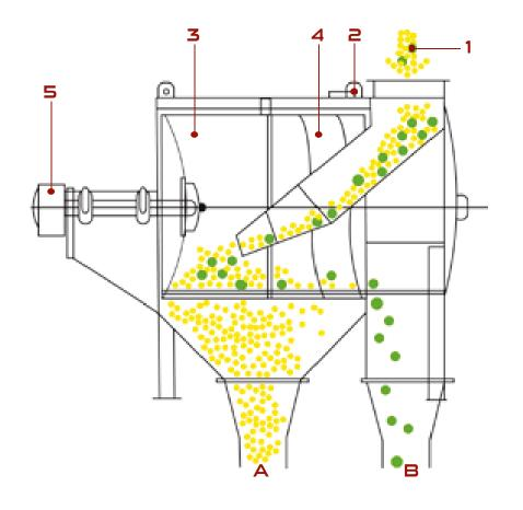
Working principle of Drum Sieve Machine
